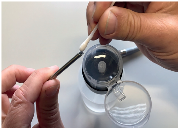
Fig. 2: Cleaning the distal end
