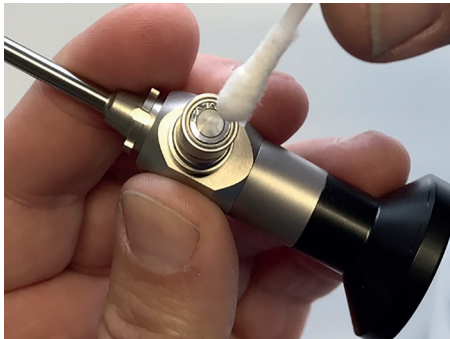
Fig. 3: Cleaning the light guide attachment
